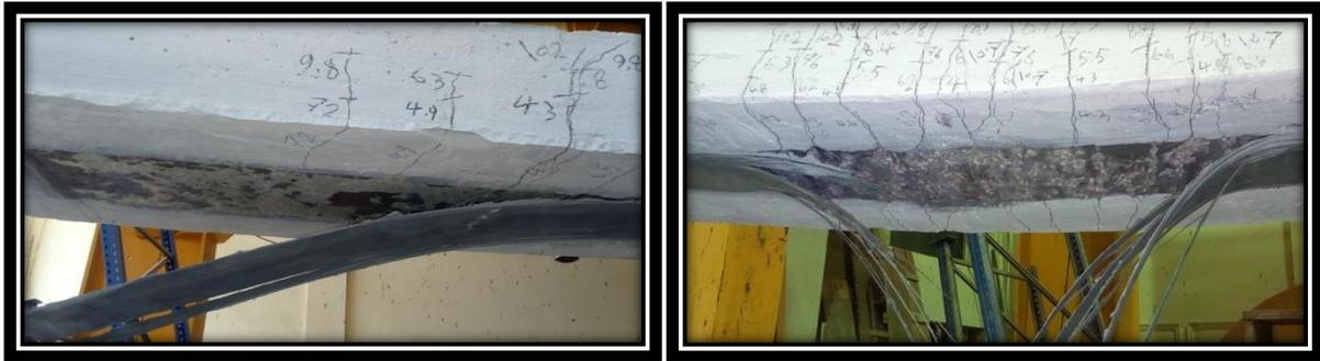
Fig. 5: The FRP debonding failure
