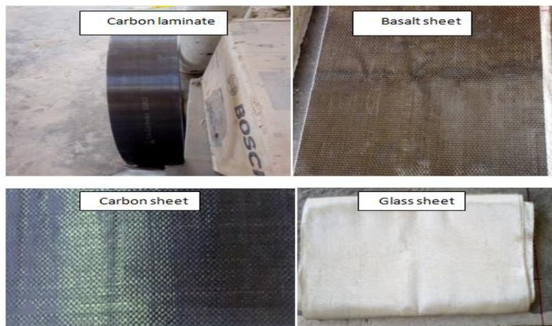
Figure 2: strengthening materials laminates and sheets used in the current study
